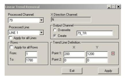
The **Processed Channel** and **Processed Line** lists show the channel and line you are currently working with. To switch to another channel and line, select them from these two lists.
