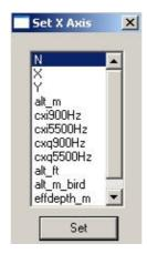
• Select a required channel in this dialog and click **Set**. The X-axis will change to the scale of the selected channel. Its label will be replaced by the name of the selected channel.
