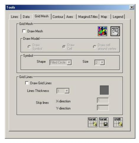
• Check **Draw Mesh** to see your grid cells filled with color (=**Show Interpolated Grid** in the **Show Layers** dropdown menu on the QC Grid toolbar). This functionality is accessible only if your data have been interpolated;
