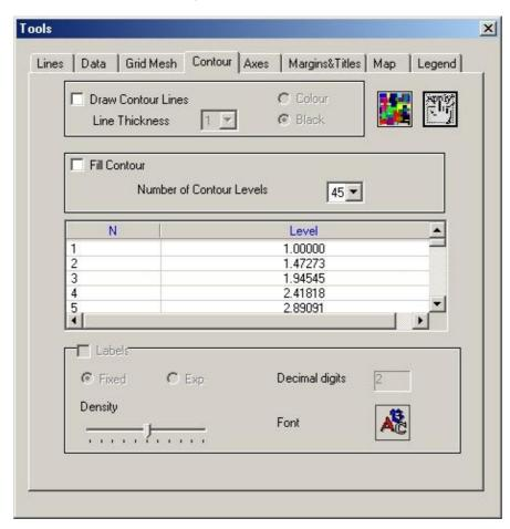
Check the Draw Contour Lines box to draw contours (=Show Contour in the Show Layers dropdown list on the QC Grid toolbar). This functionality is accessible only if your data have been interpolated; if not, a message prompts you to carry out interpolation. Click the Interpolate button and follow the steps as described in To
