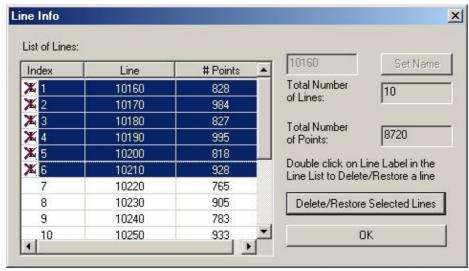
The values in the **Total Number of Lines** and **Total Number of Points** boxes in the right part of the dialog update accordingly to reflect the deletion or restoration of the line(s).
