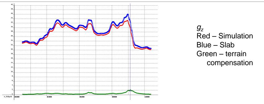
The red curve is the simulation of the .qdem grid when stations are on the topography. The density is 2 g/cm<sup>3</sup>. Blue is the bouguer slab corrections for an elevation on the topography. Green is the terrain compensation of the difference grid or theoretically the over-compensation of the slab correction.
