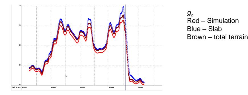
Brown is the calculated total terrain correction. The difference between red and brown is the effect of the Bouguer slab from outside the topo model to infinity. In this approach to terrain corrections, additional long grids are used to correct this virtually DC shift and extended outside radii are used to determine when the total terrain corrections converges. OR if the user only needs a relative value, the correction can be used for interpretation at this stage.
