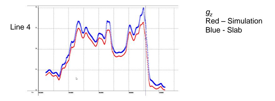
The red curve is the simulation of the .qdem grid where stations are on the topography. The 3D volume was from the surface down to GPSZ=0. The convergence of the simulation was tested up to 250,000 cells. The density is 2 g/cm<sup>3</sup>. Blue is the Bouguer slab Note: the bouguer slab corrections over-compensates for the terrain as the elevation is constant and extends to infinity.
