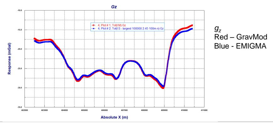
We compare the GravMod  $g_z$  value to a simulation of the topography at instrument height. We use a modern definition of Z which is upwards to be consistent with the GPS axes definitions. Thus the GravMod values are not  $g_t$  as defined classically but rather the vertical component response to the topography.
