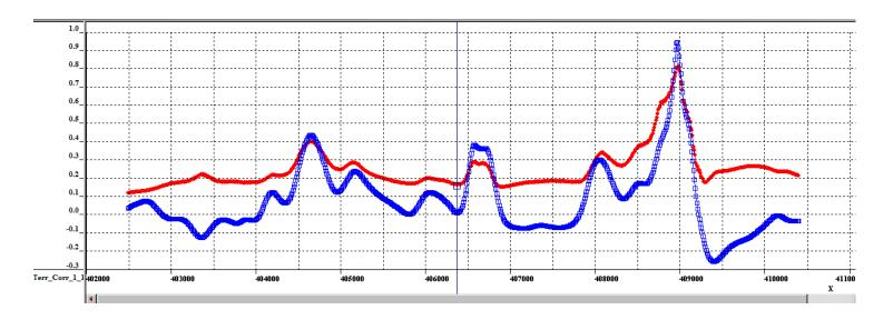
Here, we have reduced  $g_{zz}$  by a factor of 500, in order to plot  $g_t$  and  $g_{zz}$  on the same scale.
